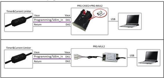
Note: PRG-MUL2 does not support "current calibration" (SDD-AAPNP supports it).
