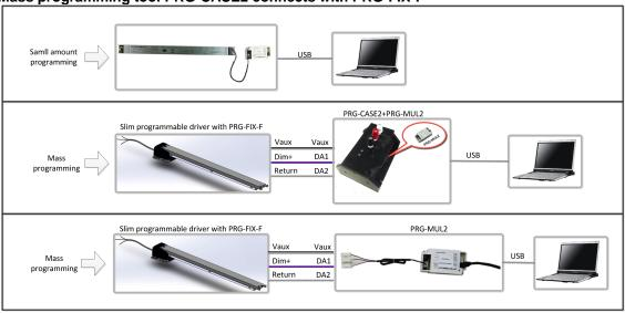
Note: Only the slim DALI driver need AC power when programming in the top diagram(Small amount programming).
