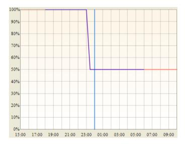
In winter the on-time should be longest, suppose 17:00 power on and 7:00 power off, the curve will be self adjust to blue wire in following picture. The transition time is same at 23:00.
