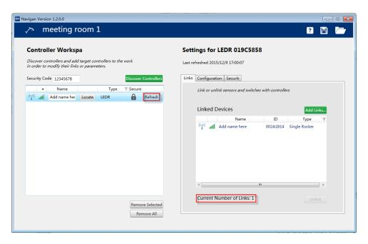
(7) Press and release the rocker switch and it will appear in the Linkable Devices list. The signal flag will blink when you click the rocker switch, select it and click "Link Selected" to finish the link operation. Now you can control the light on/off or dimming up/down by a single click or long push.
