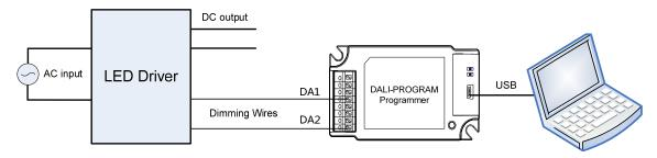
Note: The driver needs to be powered on during the programming process
