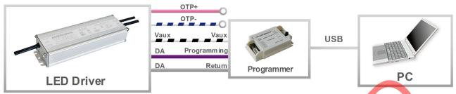
Note: (1) The driver does not need to be powered on during the programming process.
