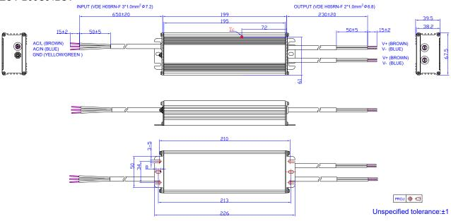
Note: The 2 DC output cables are connected in parallel internally because one 1.0mm2 wire can only carry 10A. Please connect the 2 brown wires together and 2 blue wires together in application, or ensure each cable carries same current.
