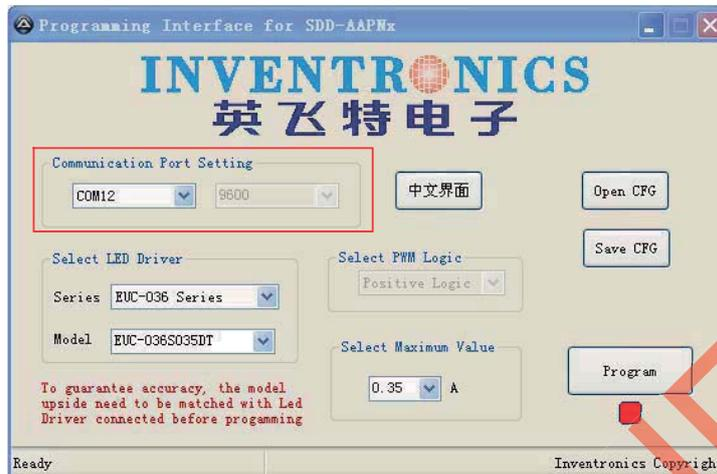
2.3.5 Select the LED driver series and model same as the one connected and set desired maximum value.
