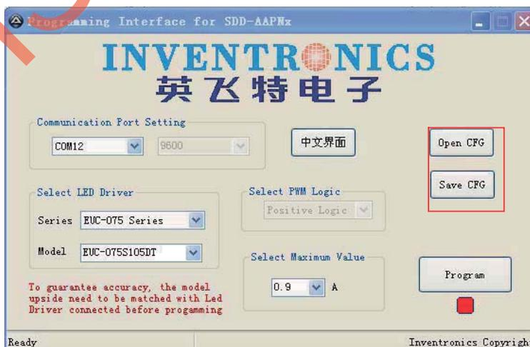
2.3.7 Click “Program” button to write the configuration to product. If there is something wrong, interface of “warning” and red indicator is shown. If programming is successful, the green indicator is shown.
