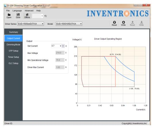
Figure 15: 0-10V Dimming Driver Configuration Window
