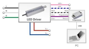
Figure 12: Programming Connections for Driver Ending in -DTA
