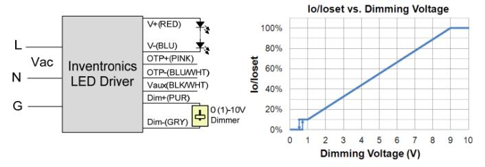
Figure 21: 0-10V Wiring and Dimming Curve
