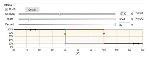
Figure 36: Internal OTP Setting
