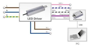
Figure 13: Programming Connections for Driver Ending in -DVA
