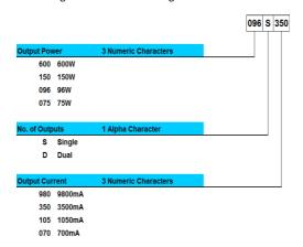
Figure 2: Part Numbering Scheme Power + Current
