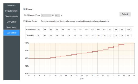
Figure 32: Output Lumen Compensation Setting
