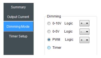
Figure 22: Selecting PWM Dimming
