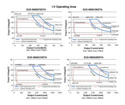
Figure 5: Specified I-V Operating Range in Datasheet
