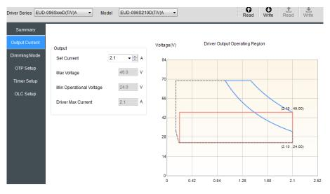
Figure 18: Software Interface Default Current Setting
