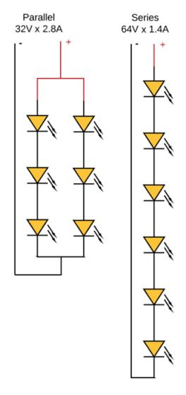
Figure 4: Example 1 in Parallel and Example 2 in Series
