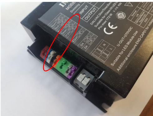
Figure 1: Example of LED drivers with auxiliary constant voltage supply
