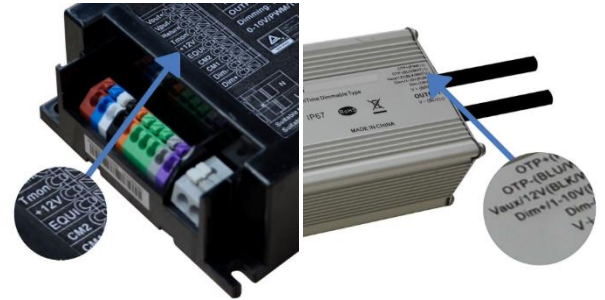
Figure 7: Example of LED drivers with auxiliary constant voltage supply
