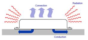
The driver case temperature, or "Tc", for safety is typically 90° C and should never be the design target for a luminaire. Instead, the luminaire should manage thermals so that the driver's worst-case, operational Tc is always maintained within the warranty specification. The luminaire's ability, *or inability*, to pull heat away from the driver will ultimately determine the life of the system.
