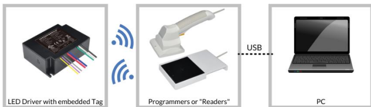
Figure 1: NFC Programming System
