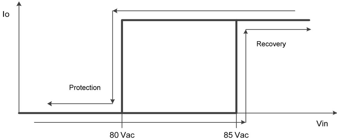
● **Input Over Voltage Protection Diagram**
