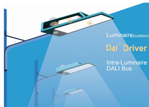
Figure 2: Intra-Luminaire Applications: DALI-2 bus does not leave the luminaire
