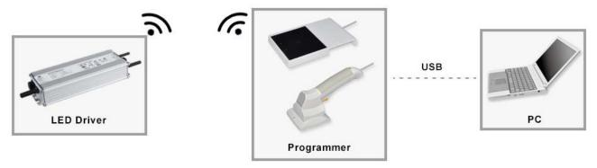
**Note:** The driver does not need to be powered on during the programming process.
