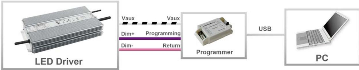
**Note:** The driver does not need to be powered on during the programming process.
