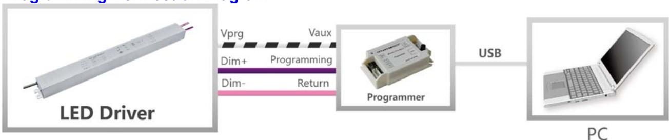
**Note:** The driver does not need to be powered on during the programming process.
