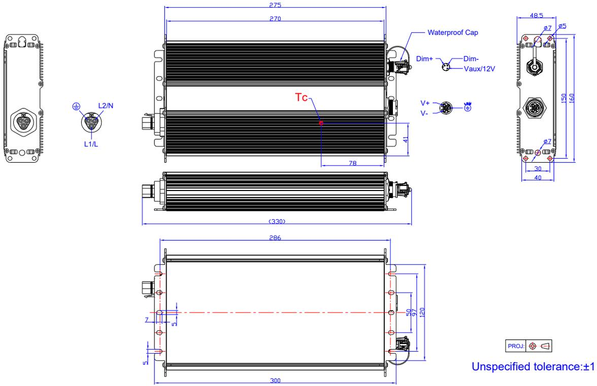
**Note:** This driver features UL Wet Location, IP67 panel mount connectors to streamline wiring in the field while still supporting stringent environmental conditions. The **mating** push-lock are not supplied by Inventronics. Please contact Wieland and Amphenol LTW or one of their suppliers for assistance sourcing the mating push-lock
