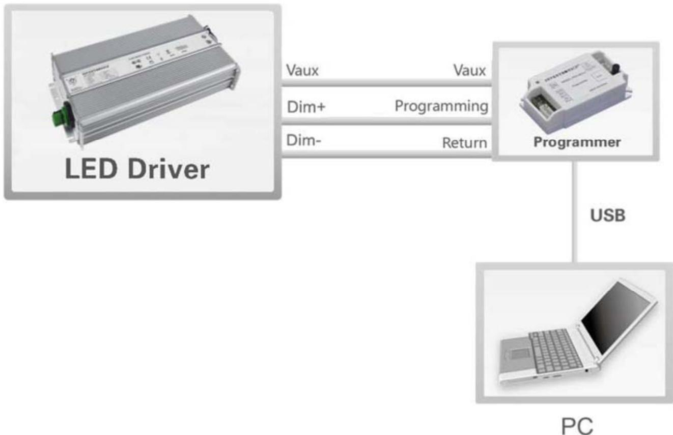
**Note:** The driver does not need to be powered on during the programming process.
