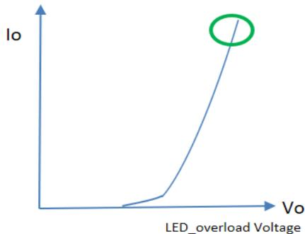
Set  $V_{overload}$  close to, but higher than the maximum forward voltage for optimized performance. The greater the difference between the  $V_{overload}$  setting and the maximum forward voltage, the higher the overload stress will be. The  $V_{overload}$  setting must be higher than  $V_f$ .
