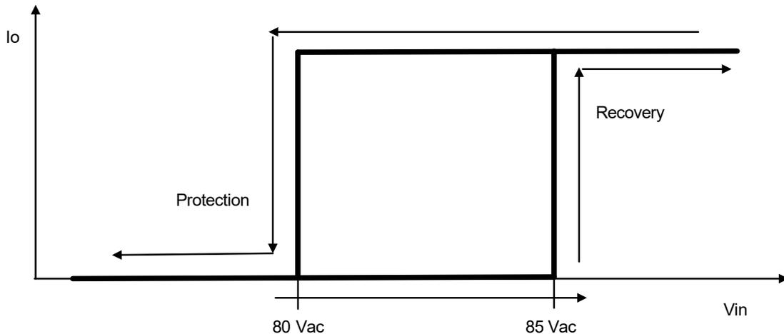
● **Input Over Voltage Protection Diagram**
