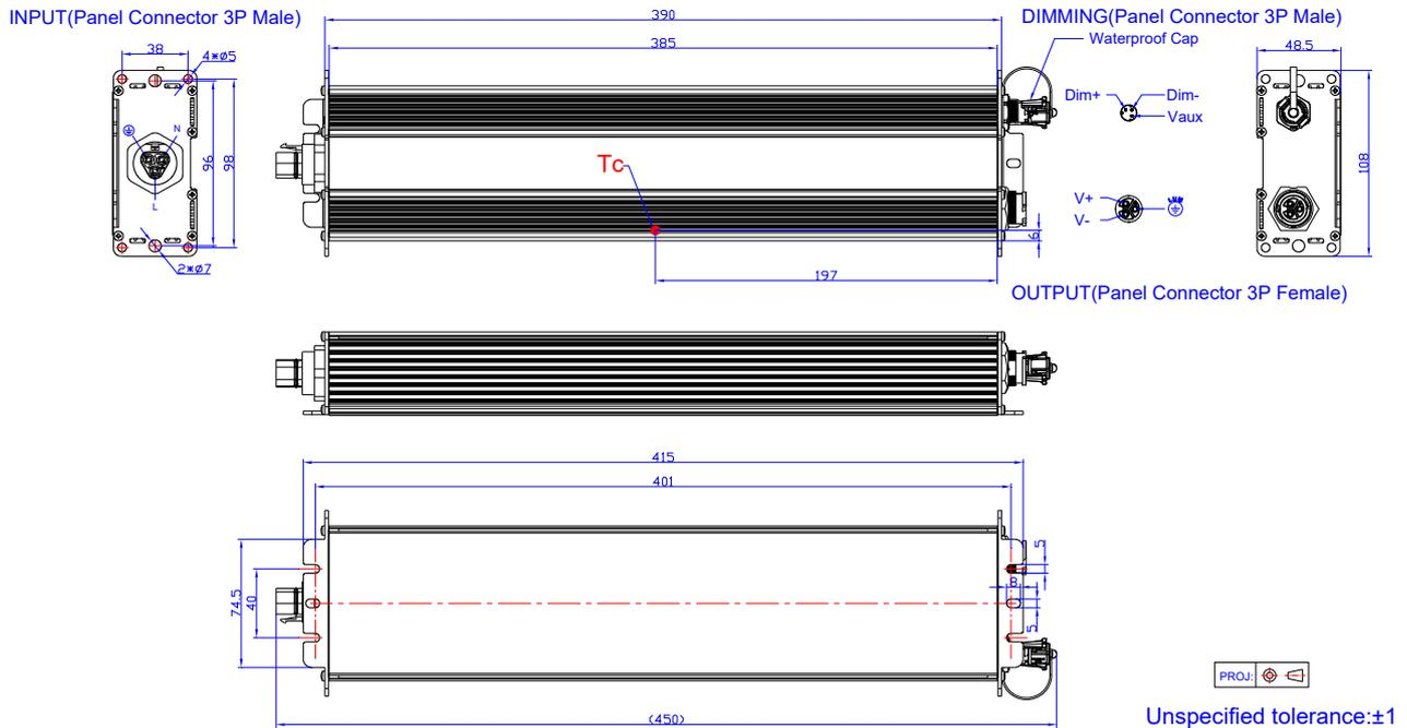
**Note:** This driver features UL Wet Location, IP67 panel mount connectors to streamline wiring in the field while still supporting stringent environmental conditions. The mating push-lock are not supplied by Inventronics. Please contact Wieland and Amphenol LTW or one of their suppliers for assistance sourcing the mating pushlock
