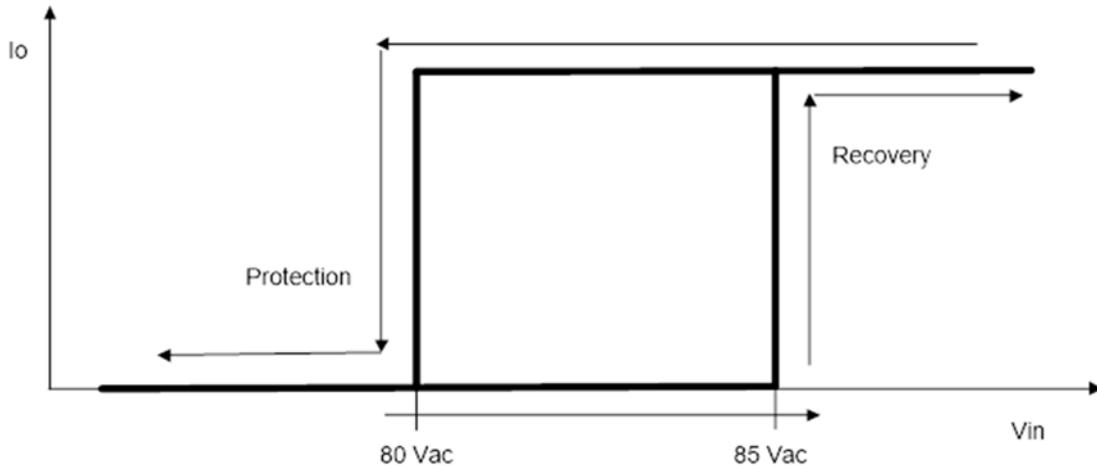
● **Input Over Voltage Protection Diagram**
