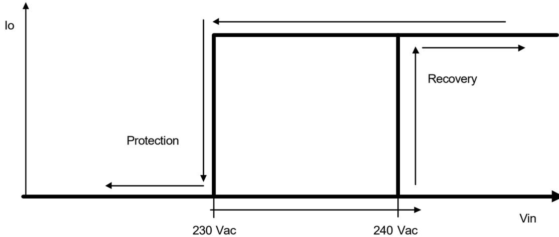
● **Input Over Voltage Protection Diagram**
