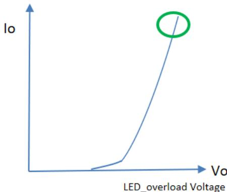
Set  $V_{overload}$  close to, but higher than the maximum forward voltage for optimized performance. The greater the difference between the  $V_{overload}$  setting and the maximum forward voltage, the higher the overload stress will be. The  $V_{overload}$  setting must be higher than  $V_f$ .
