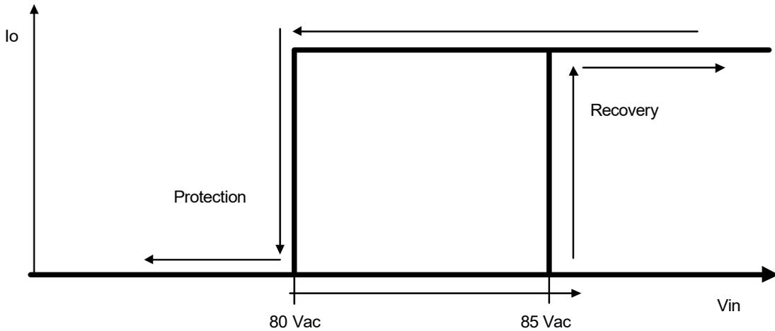
● **Input Over Voltage Protection Diagram**
