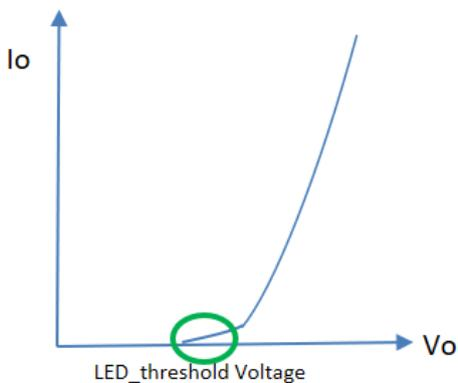
LED threshold voltage ( $V_{th}$ ) is the minimum voltage required for current to flow through the LED load. After this threshold is met, the LED forward voltage ( $V_f$ ) increases as the current increases.
