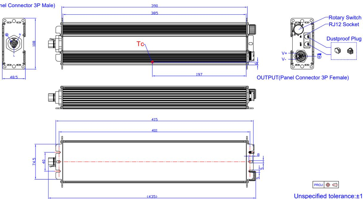
**Note:** This driver features UL Wet Location, IP66 panel mount connectors to streamline wiring in the field while still supporting stringent environmental conditions. The mating push-lock are not supplied by Inventronics. Please contact Wieland and Amphenol LTW or one of their suppliers for assistance sourcing the mating push-lock.
