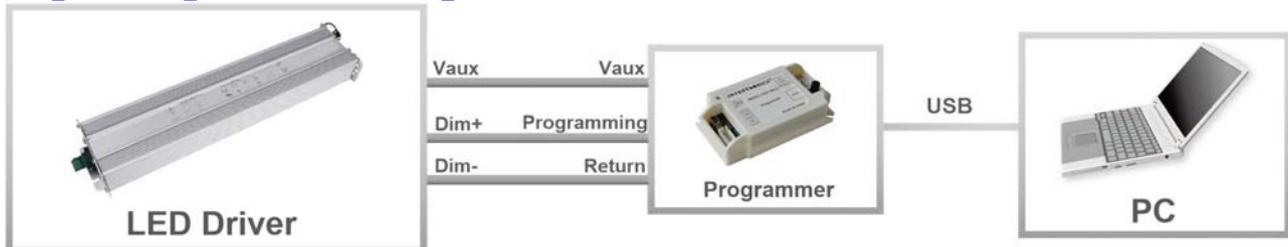
**Note:** The driver does not need to be powered on during the programming process.
