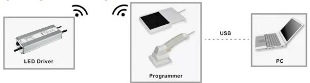
Note: The driver does not need to be powered on during the programming process.
