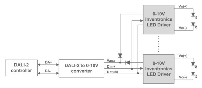
**Note:** Normally the converter is powered by 1 driver. If the converter is powered by more than 1 driver, each Vaux line should have a diode mounted to prevent current streaming between the drivers, because current streaming may cause dimming failure.
