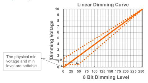
**Note:** (1) The logarithmic dimming curve can be modified in the same way.
