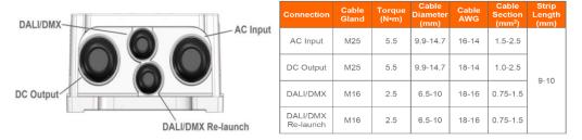
Note: All gland connectors should be used during field operation. Larger sealings are available on request.
